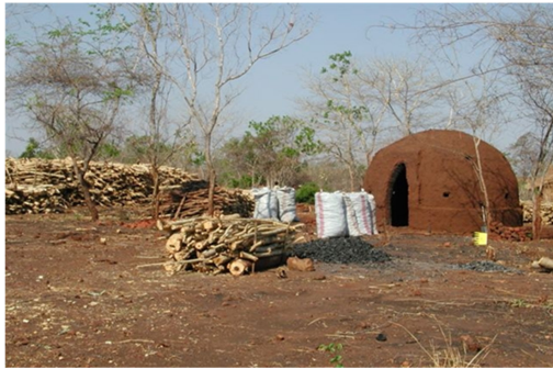
Figure 12.125: Carbonisation using Half Orange kiln
