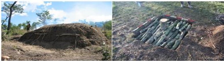
Figure 1114 Earth-mound and pit kilns
